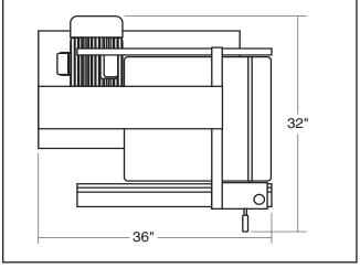
Figure 12. G0514 minimum working clearances.
